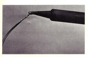
Photo 1. After stripping about 3/8 inch of insulation from each wire, apply an even coating of solder.
